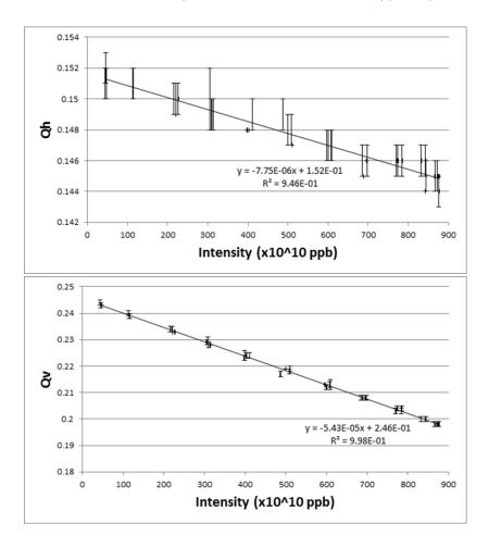
There is a good linear response of Q to intensity and the results are consistent with previous measurements and the impedance model.
